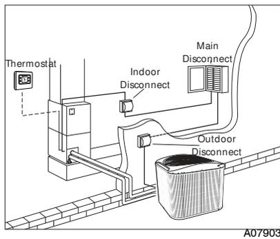
Fig. 1 - Electrical Disconnects
